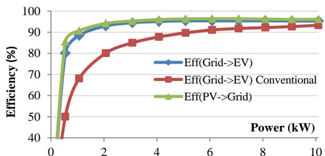
Fig. 4. Measured efficiency of the converter for PV→Grid, EV→Grid
