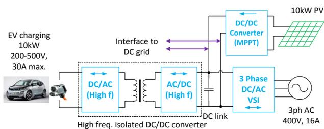
Fig. 3. Topology of power converter (top) and 10kW prototype of developed converter compared to a conventional PV inverter and EV charger (bottom)
