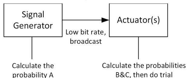
Fig. 1. Basic mechanism of low bit rate broadcast
