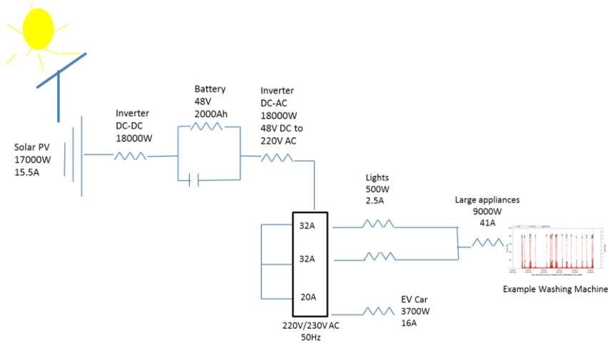
Figure 2 Off-grid circuit description for a house in Nunspeet-the Netherlands, using a battery as principal power.
