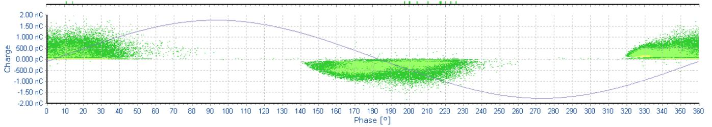
Fig. 1. Pattern diagram for partial discharges under 4.5 kV rms ac conditions.
