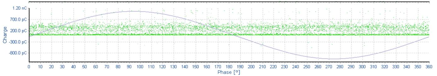
Fig. 2. Pattern diagram for partial discharges under 6.6 kV dc conditions.
