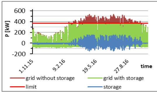
Fig. 1: Operation of battery for peak shaving in a pilot [6]
